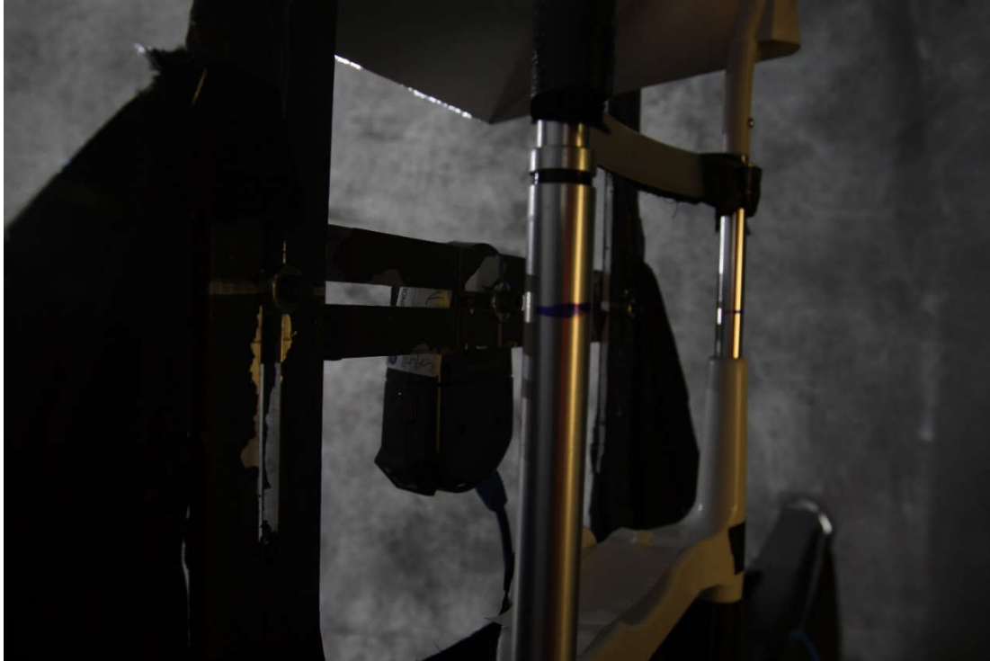
Figure 3-57. Illuminance meter installed on the bar at the eye level (close-up)
