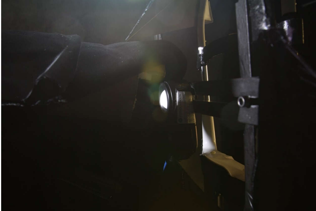
Figure 3-64. Illuminance meter is in “full” view of the glare source (no shadows)
