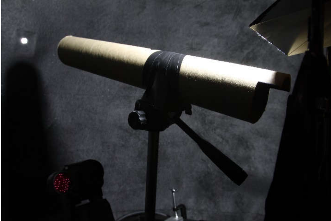
Figure 3-60. Tube for measuring the direct illuminance component from the glare source
