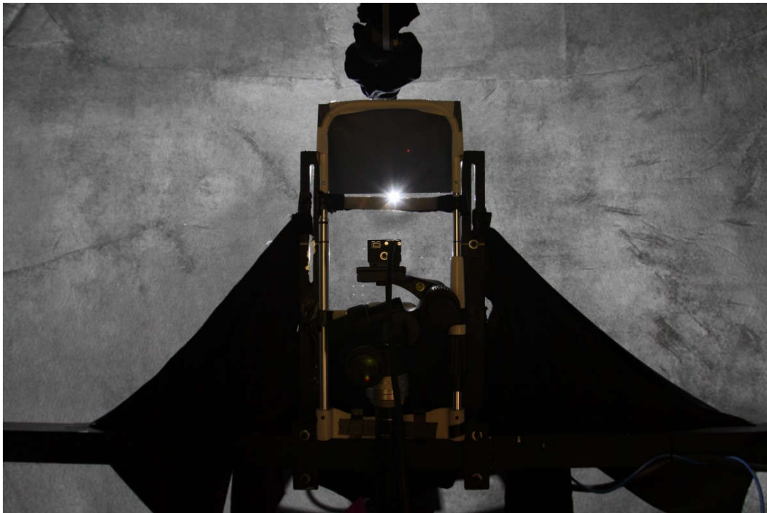
Figure 3-65. Luminance mapping camera (at the eye level) used for checking the aiming of the glare sources
