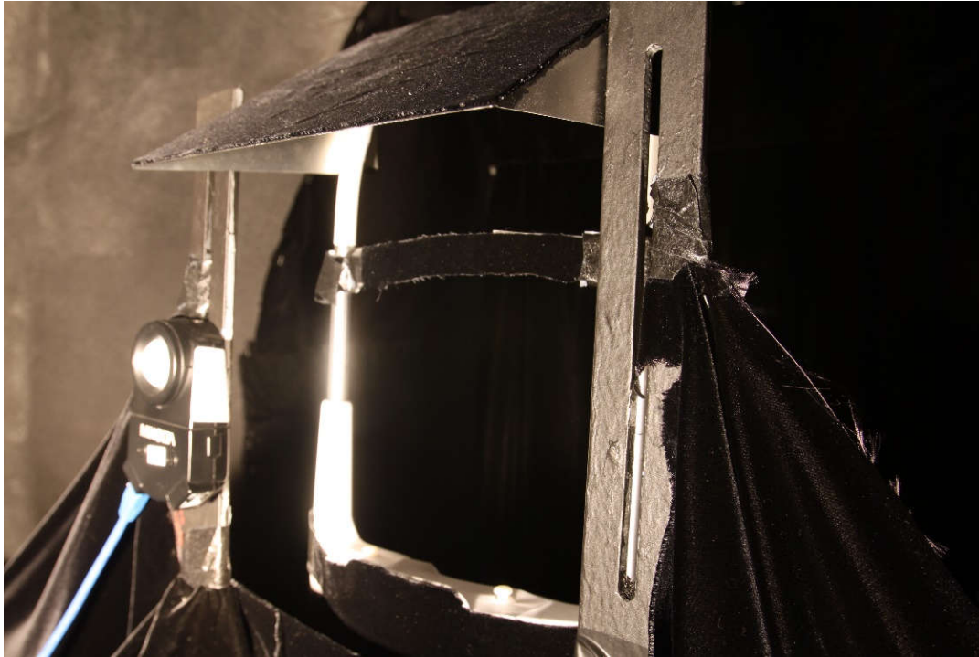
Figure 3-14. Chinrest and the screen covered with black velvet ( \rho=0.006 )
