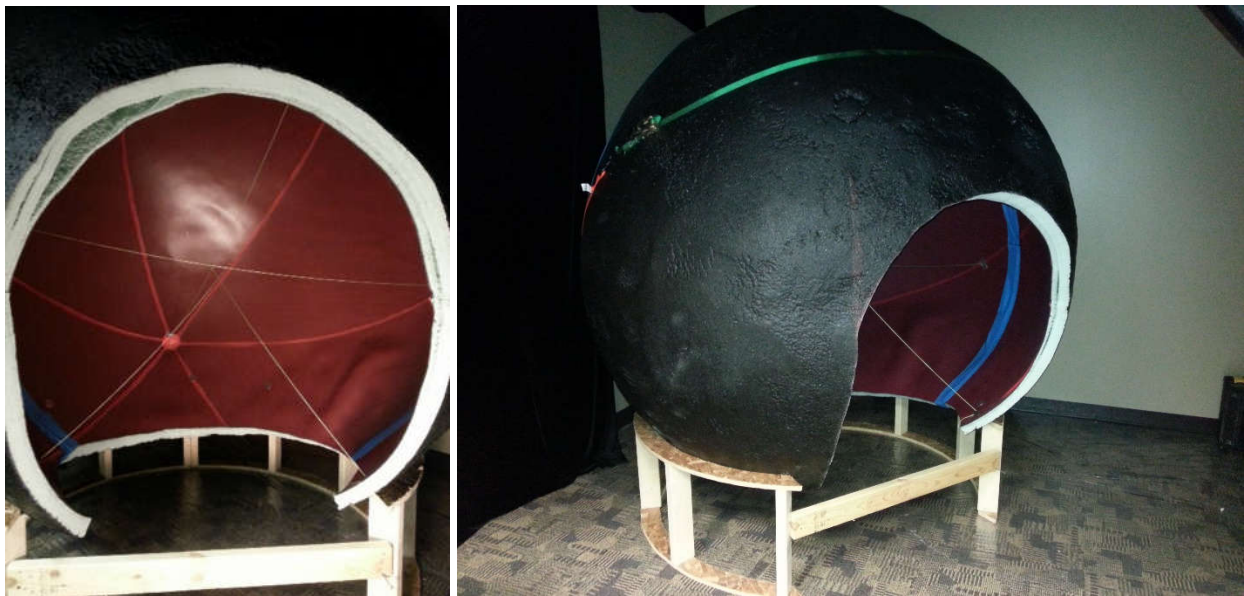
Figure 3-8. Core of the sphere made from a helium parade balloon (left), sphere during the early stages of construction (right)
